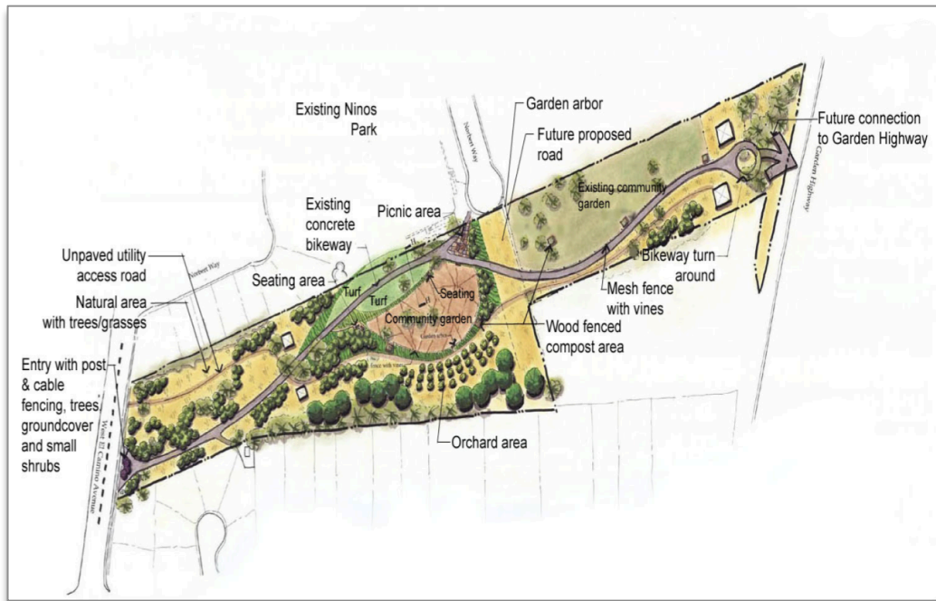
Figure 9. Niños Park Bikeway Master Plan, Section 4. From report to City Council on the Ninos Parkway Project, Phase Three (August 17, 2010). Plan shows proposed clearance area under the towers, utility access road, extended bike path into existing garden, and new community garden adjacent to the International Garden of Many Colors.
